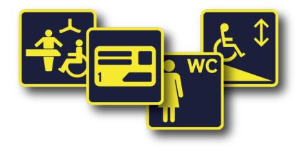
Clear, bold and intuitive iconography to highlight the location of key features around the station. The use of a standard format with high colour contrast means that these features can be easily located with little effort by passengers.
